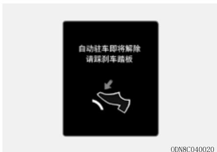
**自动驻车(AUTO HOLD)关闭! 踩下制动踏板**
